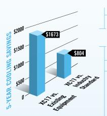
SEER stands for "Seasonal Energy Efficiency Ratio" and is a measure of the cooling efficiency of air conditioners. The higher the SEER, the greater your energy savings. Typical SEER ratings start at 13.00, but the XC17 carries ratings as high as 18.00.
